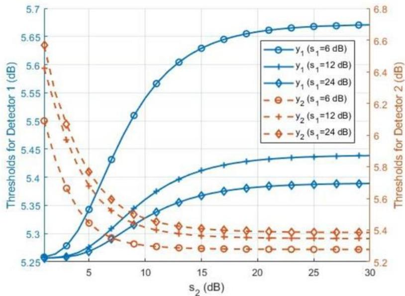
*Result of optimizing the local detection thresholds for the OR rule.*
